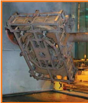
Water bath cool down process
